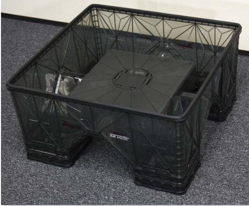
2. Hold the canvas hood in place by its top over the SAH with the Dwyer trademark facing you and place the adapter hood into the main SAH body aligning the sewn corner seams of the adapter hood to be approximately in line with the corner of the SAH unit body to prepare for assembling it to the SAH body as shown below.
