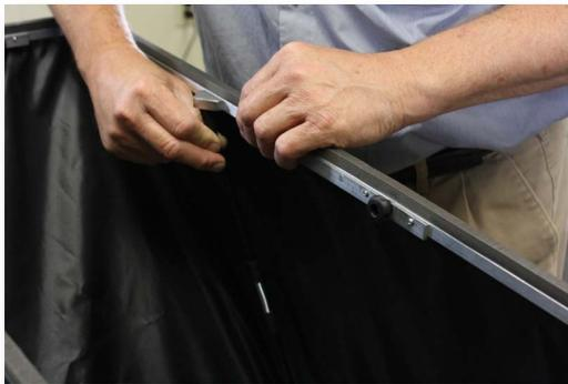
12. Re-tuck the upper cord loop into the top frame if it came free during the assembly. At this time, you can tuck the outer lower cord into the SAH unit along the straight sections. It is not necessary that this be done for the cord to stay in place or for the system to perform properly.
